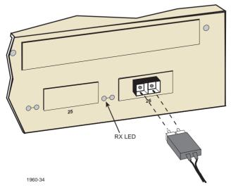
Figure 3-11 FE-100FX and FE-100F3 Ports
